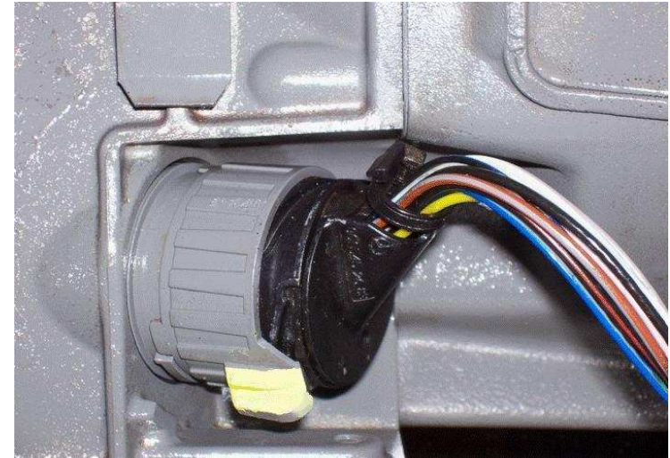
Harness plugged in, lock tab must be twisted clockwise to secure properly.
