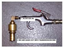
2. Manually check the modulator by using shop air to the inlet side of the modulator. There should not be any air leakage from the transmission side of the modulator.
