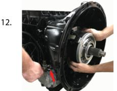
Install the air line and electrical connector to clutch control valve.
