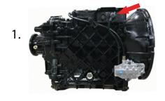
Disconnect the clutch valve wiring connector at the control housing.
